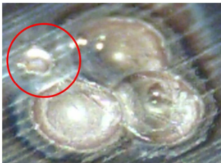
Electrode contamination can lead to small “explosions” that create craters in the workpiece. All four welds were made at the same setting. Metal contamination on the electrode caused one weld to create a crater.
