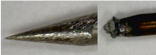
Electrode condition greatly affects energy transfer and also weld properties (see above discussions). Left: A perfect electrode. Right: An electrode in poor condition with metal contamination.
